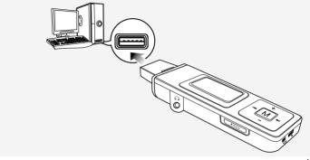
Remove the USB Cover then connect the USB Connection Plug to the USB port (  $\sqrt[4]{y}$  ) on your PC.
